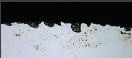
Ground PCD cutting edge Diamond grains that are torn out leave gaps in the microstructure and produce chipping. Microstructure close to cutting edges is also damaged by grinding pressure.
