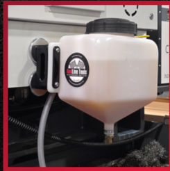
COOLANT MIXING STATION
