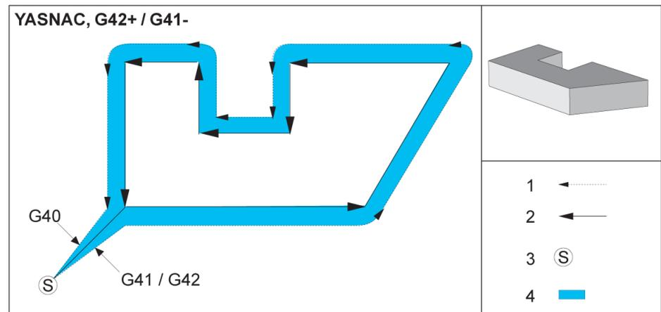
**Cutter Compensation, FANUC Style, G41 with a Positive Tool Diameter or G42 with a Negative Tool Diameter:**
