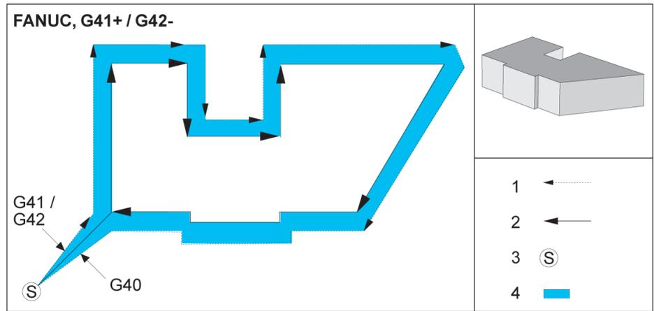
**Cutter Compensation, FANUC Style, G42 with a Positive Tool Diameter or G41 with a Negative Tool Diameter:**
