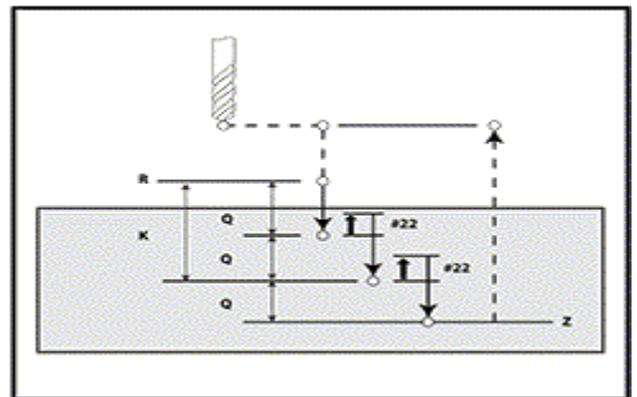
If only *Q* is specified, a different operating mode is selected for this canned cycle. In this mode, the tool is returned to the *R* plane after all pecks are completed, and all pecks will be equal to the *Q* value.
