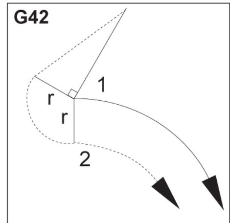
**Cutter Compensation Entry (Fanuc style) Type A and B:**
