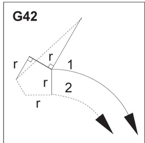
**Circular Interpolation and Cutter Compensation**
