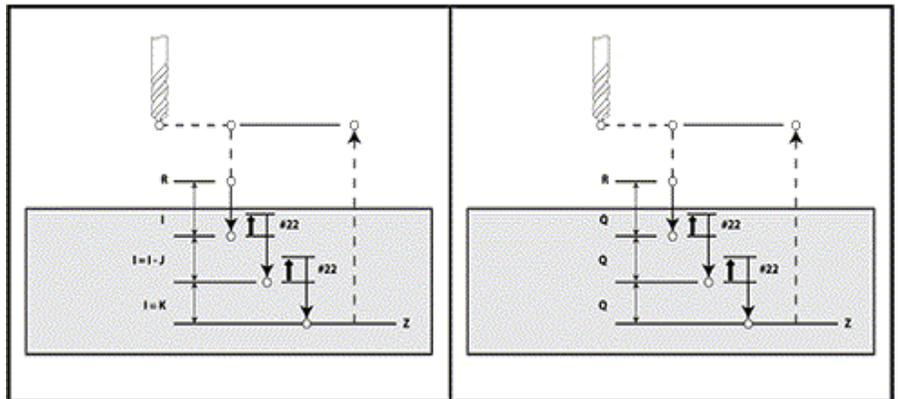
If *I*, *J*, and *K* are specified, The first pass will cut in by the value *I*, each succeeding cut will be reduced by the value of *J*, and the minimum cutting depth is *K*. If *P* is specified, the tool will pause at the bottom of the hole for that amount of time.
