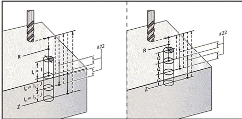
Setting 52 changes the way G83 works when it returns to the R plane. Usually the R plane is set well above the cut to ensure that the peck motion allows the chips to get out of the hole. This wastes time as the drill starts by drilling empty space. If Setting 52 is set to the distance required to clear chips, you can set the R plane much closer to the part. When the chip-clearing move to R occurs, Setting 52 determines the Z-Axis distance above R.
