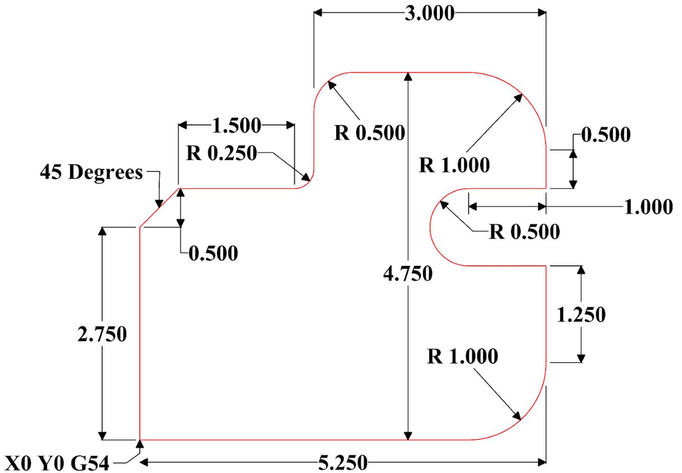
**Program Tool Path Using any Method. G01 w/ ,R#.#, G02, or G03. Incremental or Absolute.**
