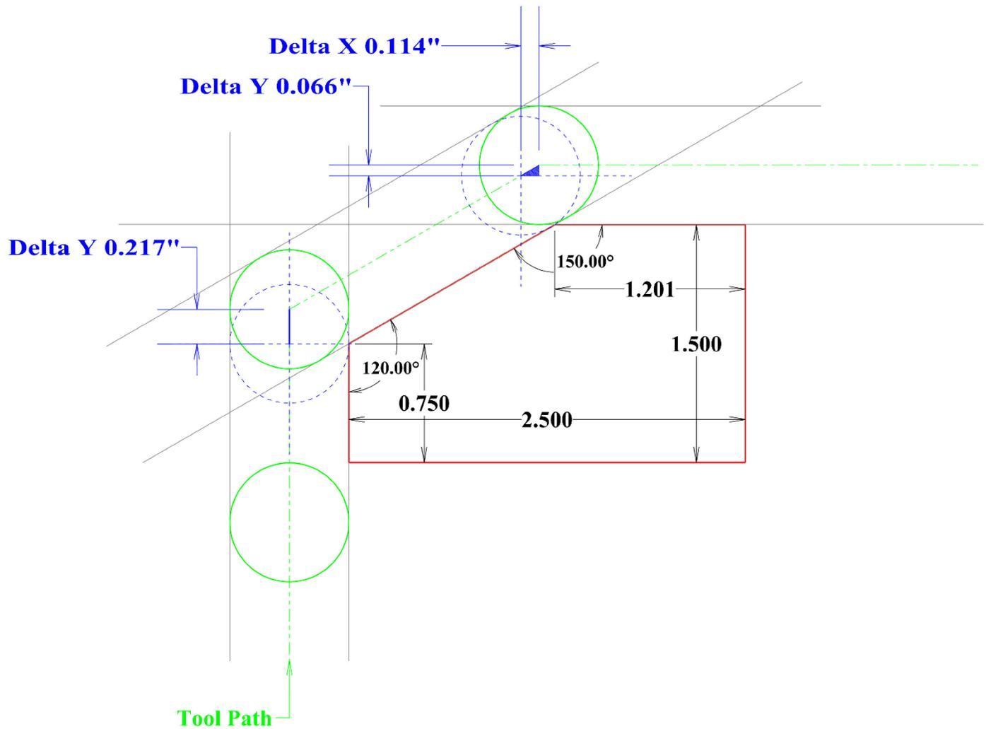
The Tool Path above requires additional calculation for **0.75"** Diameter Tool.
