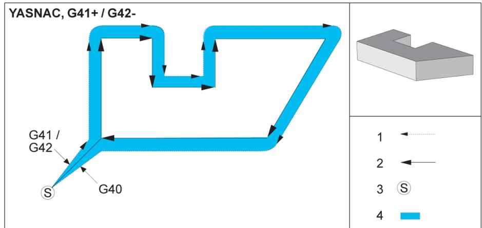
**Cutter Compensation, YASNAC Style, G42 with a Positive Tool Diameter or G41 with a Negative Tool Diameter:**
