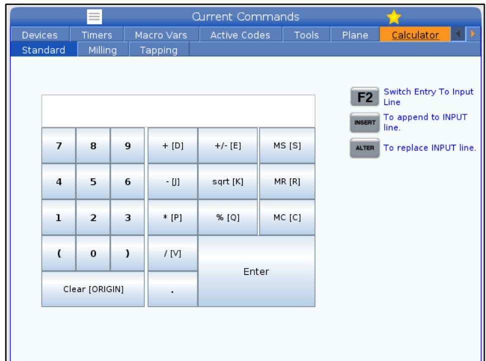
To insert an arithmetic operator, use the letter key that appears in brackets next to the operator you want to insert.
