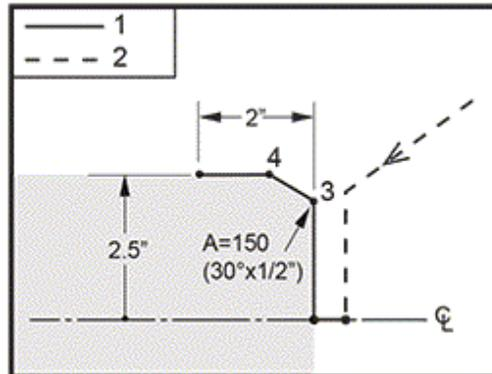
\*\*\* Program on USB Drive; G01 LINEAR INTERPOLATION MOTION (GROUP 01)\O60012 (Chamfering).NC \*\*\*
