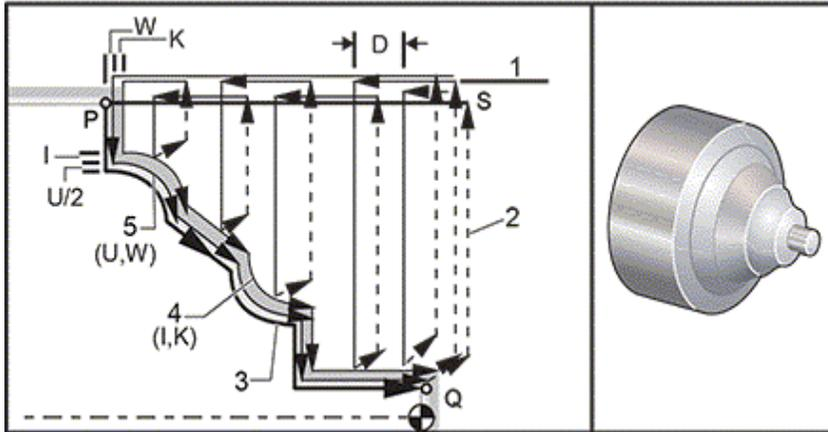
The G72 consists of a roughing phase and a finishing phase. The roughing and finishing phase are handled differently for Type 1 and Type 2. Generally the roughing phase consists of repeated passes along the X-axis at the specified feed rate. The finishing phase consists of a pass along the programmed tool path to remove excess material left by the roughing phase while leaving material for a G70 finishing cycle. The final motion in either type is a return to the starting position S.
