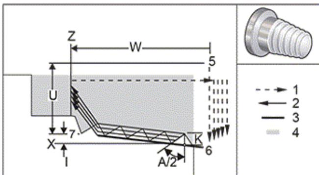
The G76 canned cycle can be used for threading both straight or tapered (pipe) threads.
