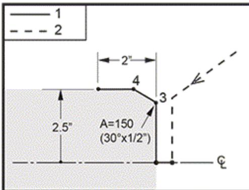
\*\*\* Program on USB Drive; G01 LINEAR INTERPOLATION MOTION (GROUP 01)\O60012 (Chamfering with 'A').NC \*\*\*
