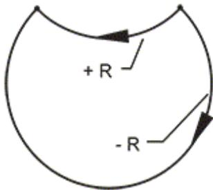
$I$  and  $K$  are used to specify the center of the arc. When  $I$  and  $K$  are used,  $R$  may not be used. The  $I$  or  $K$  is the signed distance from the starting point to the center of the circle. If only one of  $I$  or  $K$  is specified, the other is assumed to be zero.
