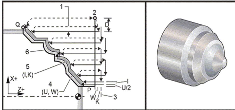
This canned cycle roughs material on a part given the finished part shape. Define the shape of a part by programming the finished tool path and then use the G71 PQ block. Any F,S or T commands on the G71 line or in effect at the time of the G71 is used throughout the G71 roughing cycle. Usually a G70 call to the same PQ block definition is used to finish the shape.
