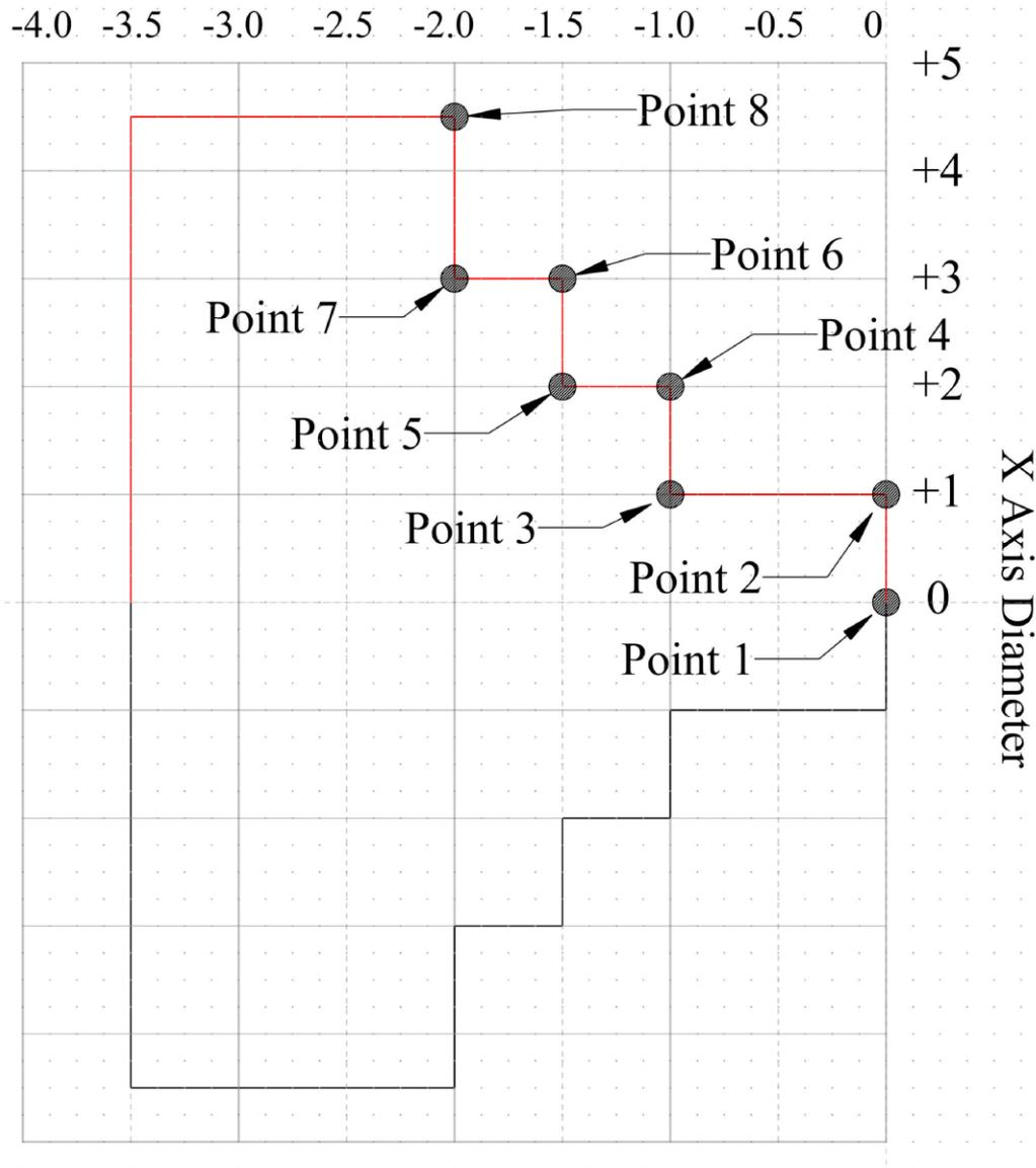
Starting from X0, Z0 to point 5. Fill in the tool path positions below for both absolute and incremental movements.
