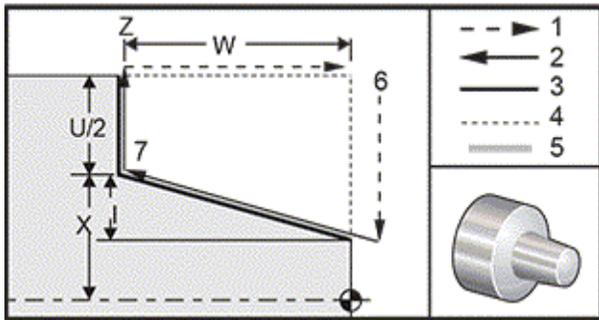
G90 is used for simple turning, however, multiple passes are possible by specifying the *X* locations of additional passes.
