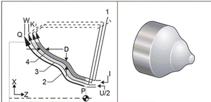
The *G73* canned cycle can be used for rough cutting of preformed material such as castings. The canned cycle assumes that material has been relieved or is missing a certain known distance from the programmed tool path *PQ*.
