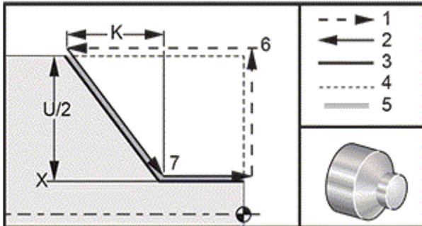
Straight end facing cuts can be made by specifying  $X$ ,  $Z$  and  $F$ . By adding  $K$  a cone-shaped face is cut. The amount of coning is referenced from the target. That is  $K$  is added to the value of  $X$  at the target. Any of the four ZX quadrants is programmed by varying  $U$ ,  $W$ ,  $X$ , and  $Z$ . The coning is positive or negative. The following figure gives a few examples of the values required for machining in each of the four quadrants.
