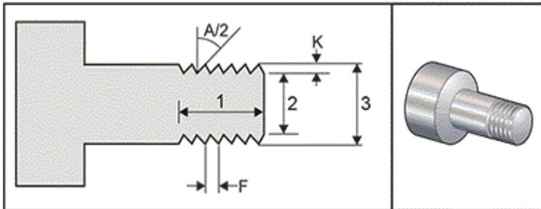
Setting 95/Setting 96 determine chamfer size/angle; M23/M24 turn chamfering ON/ OFF.
