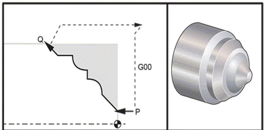
The G70 cycle is like a local subprogram call. However, the G70 requires that a beginning block number (P code) and an ending block number (Q code) be specified.
