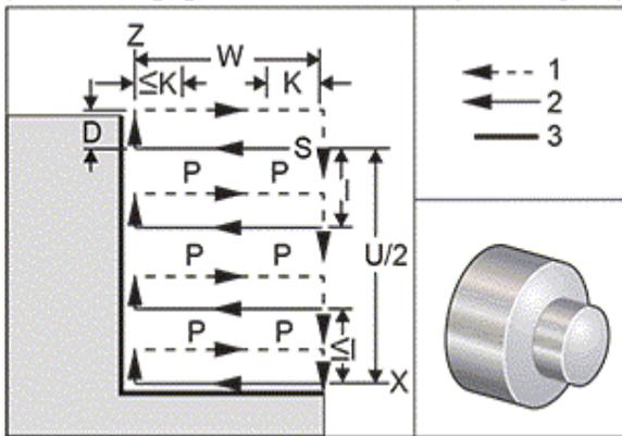
The G74 canned cycle is used for grooving on the face of a part, peck drilling, or turning.
