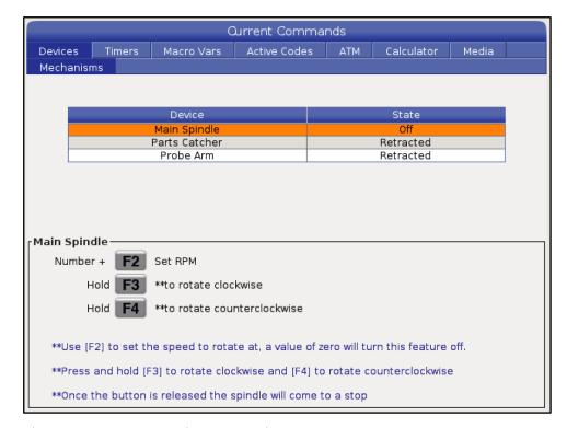
down **[F4]** to rotate the spindle counterclockwise. The spindle comes to a stop when the button is released.
