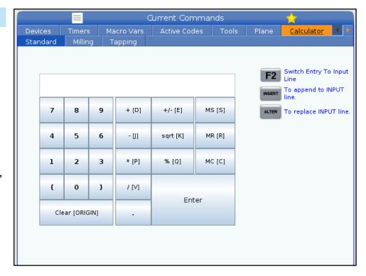
multiplication, and division, as well as square root and percentage. The calculator lets you easily transfer operations and results to the input line so that you can put them into programs. You can also transfer results into the Milling and Tapping calculators.
