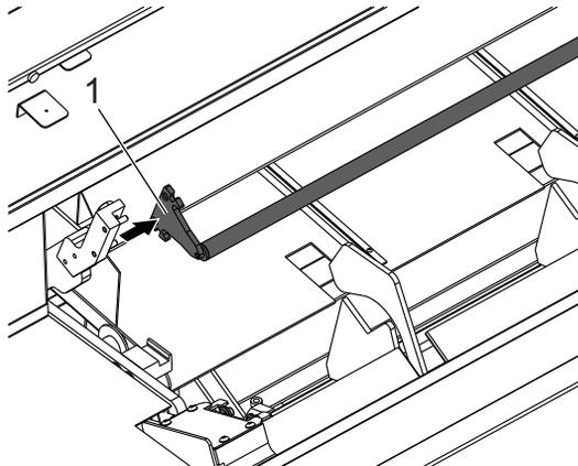
4. Remove the push rod and bushing. Follow this procedure in reverse to install the other push rod.
