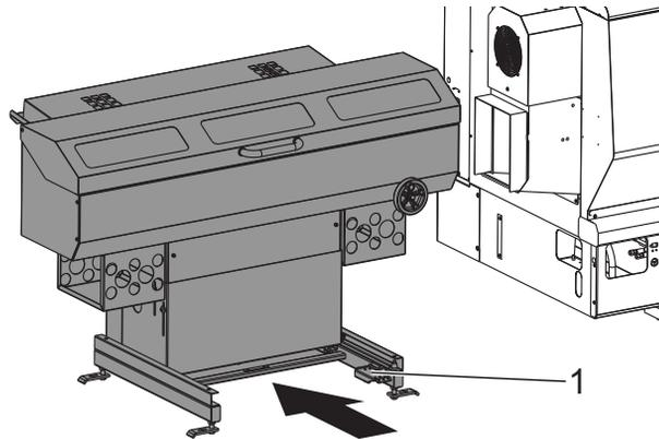
**Lockout / Lathe Setup Position:** Press the release pedal [1] at the base, and then push the Bar Feeder back. This mode disables all Bar Feeder motion. With the Bar Feeder in this position, you have easy access to change spindle liners, clean the coolant collector, or do other tasks on the lathe spindle.
