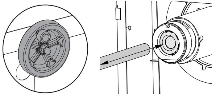
4. Use the wheel to adjust the transfer tray height. Turn it clockwise to raise the tray and counterclockwise to lower the tray. As you adjust the transfer tray height, move the bar into the spindle liner by hand. Continue to adjust the transfer tray height until the bar slides freely into the liner.
