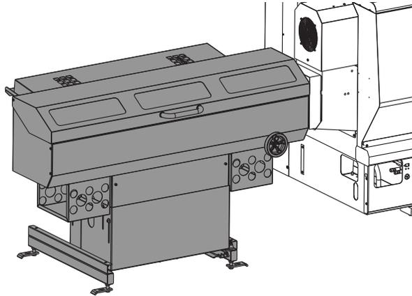
**Feed / Auto Position:** This is the Bar Feeder's normal operating position. You can command Bar Feeder motion at reduced speed with the lid open. In this position, you can set up your bar feed application, check and adjust tray height alignment, and run your application.
