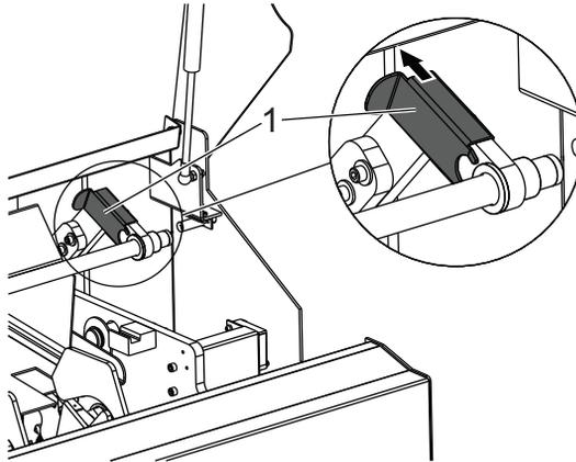
3. At the other end of the push rod, pull the retention blade off of the holder block.
