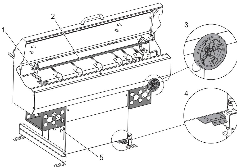
**1. High-Speed, Belt-Driven Bar Pusher:** This mechanism quickly, smoothly, and accurately feeds bar stock into your lathe.
