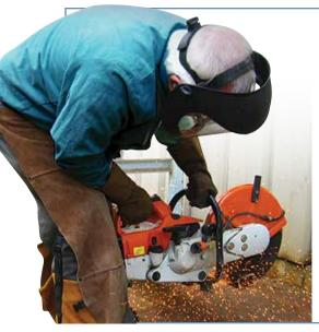
Norton high-speed cut-off abrasive wheels provide the industry's leading performance in all high-speed gas and electric-powered applications.
