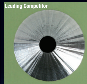
Chatter generates a rough finish for inferior fastener fitment.
