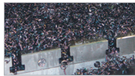
T-slots packed with difficult to remove chips
