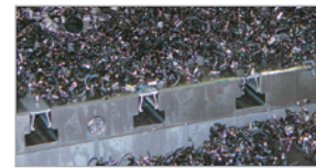
T-slots protected & clear by T-Slot Clean
