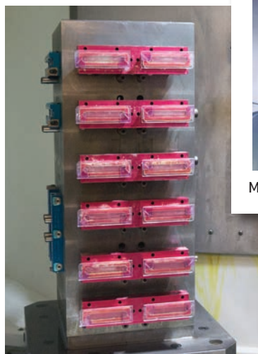
DoveLock jaws used for glass machining
