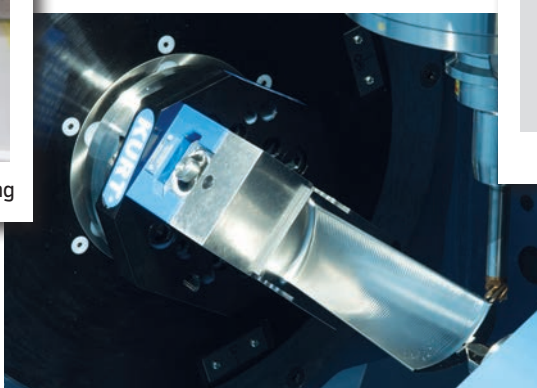
MaxLock 5 axis vise used for turbine blade machining
