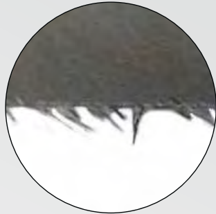
Typical delamination on a milled CFC workpiece edge
