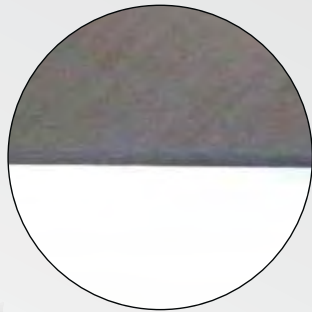
Milled CFC workpiece edge without delamination machined with a Guhring CR 100 end mill
