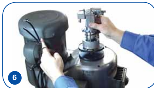
6 Position powerhead and secure with socket head cap screws [SHCS].
