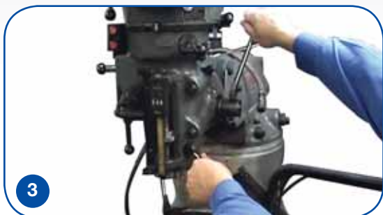
3 Return quill to upper position and lock break.
