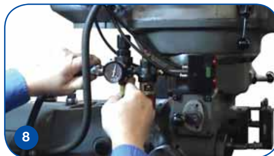
8 Hook up shop air and adjust regulator to 80-90 psi.
