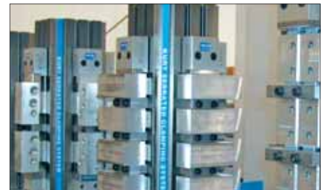
Solution: Kurt serrated Double Station vise towers on palletized machining centers for 24/7 production.
