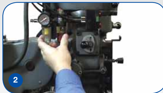
2 Place the switch and secure with socket head cap screws [SHCS].
