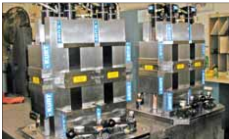
Solution: Multiple towers with DoubleLock vises on palletized machining center for 24/7 production.
