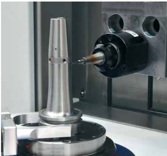
Automated correction of unbalance via CNC machining unit
