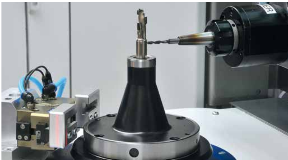
Balancing of tools with a HG balancing adapter for tools with a cylindrical shank
