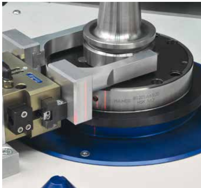
Integrated balancing adapter and gripper for automatic index measuring
