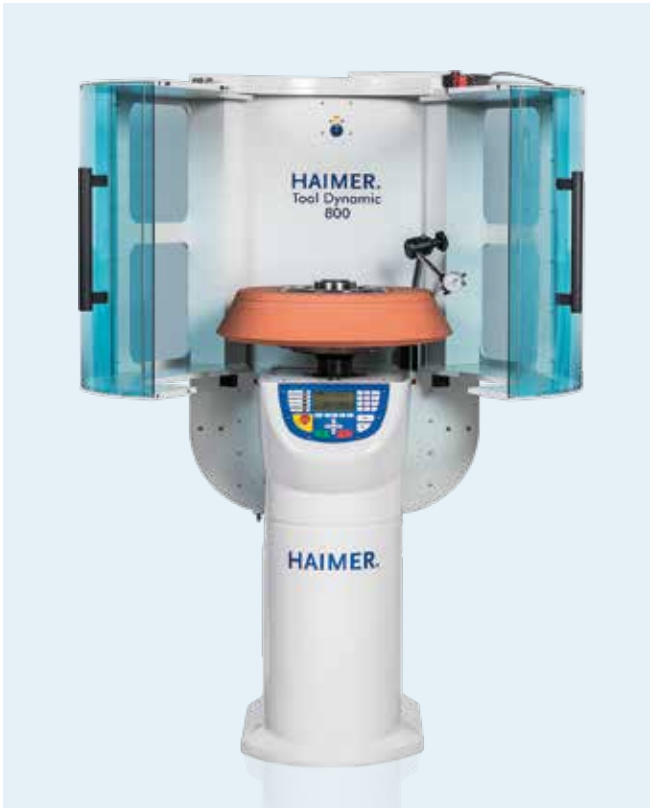
The safety hood is segmented and opens to the side. Thus the rotor is accessible from above. Heavy parts can be handled by a crane.
