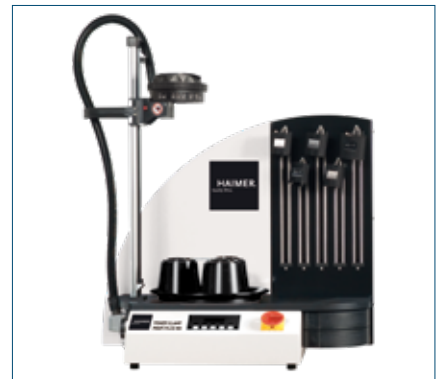
Power Clamp Profi Plus NG High powered shrink fit machine – Heating power 20 kW – For shrinking of tools from Ø 1/8"–2" (3–50 mm) – For HSS- and solid carbide tools – Big coil for Ø 1½"–2" (40–50 mm) optional – Incl. rotary table and chuck support – Incl. tool tray – With craning boxes for accessories
