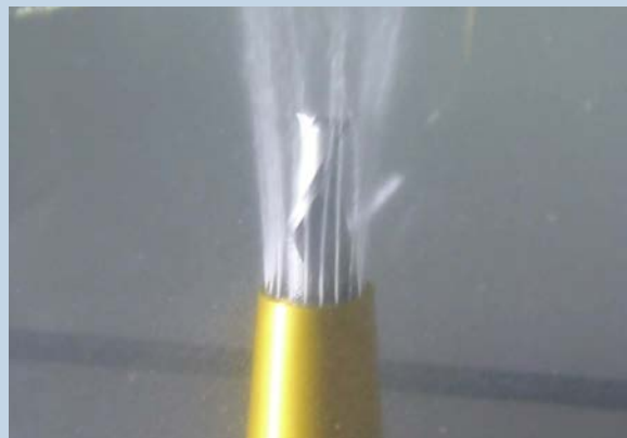
Slip-on sleeve with nozzles – ineffective cooling, coolant does not reach the cutting edges
