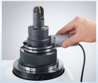
Manual positioning of the read/write head
