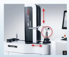
Second camera for presetting the center of rotation (optional)
