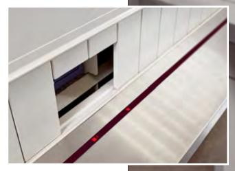
The compartment indicator shows where the article can be retrieved. These compartment doors open automatically
