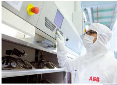
Storage of contamination-sensitive products up to clean-room class 5 according to DIN EN ISO 14644-1
