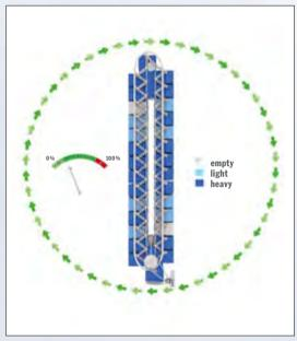
When the load is evenly distributed in the Hänel Rotomat® very little energy is required for the rotation movement
