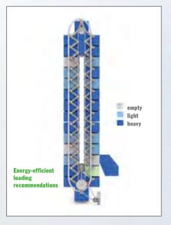
Weight distribution in the Hänel Rotomat\* is measured continuously so that if a load becomes uneven, a relocation of goods is recommended by the Hänel EcoLoad\* warning device to optimize energy efficiency
