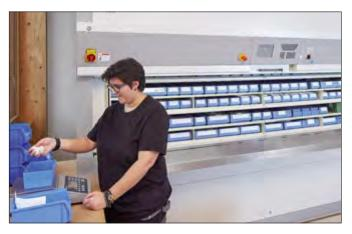
Loose parts are counted by weight on a scale near the storage system and then delivered to the assembly area
