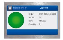
The web device indicates which bin to use for the picking process. Retrieval is confirmed using the web device
