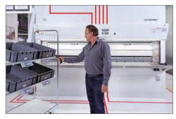
The picking bins are allocated with a barcode scanner
