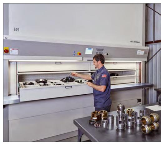
Safe and secure storage of heavy components in the Hänel Rotomat®
