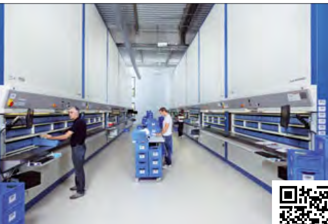
Small parts are picked quickly and efficiently from 12 Hänel Rotomat® storage carousels
