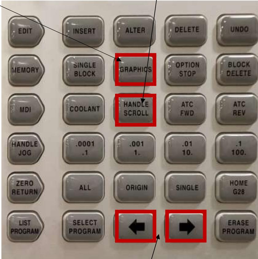
The [SEND] AND [REC] KEYS have been changed to FORWARD and BACK KEYS.
