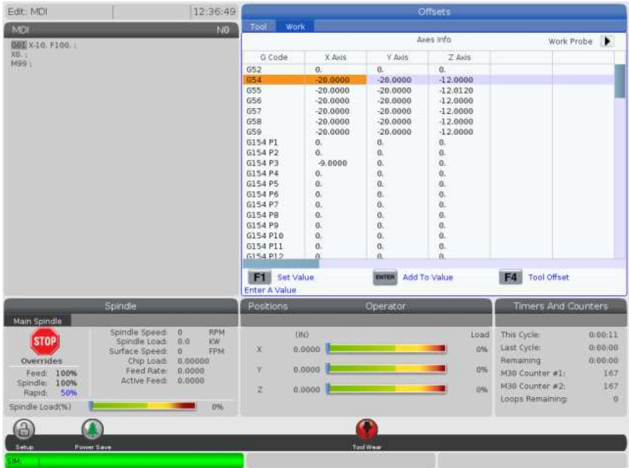
**[Current Commands] key** gives many different options. Note the **Timers** tab is highlighted. On this page current date and time, cycle time, M30 counters for keeping track of the number of parts and Macro values may be indicated. One may cursor down into the page to reset the M30 counter by pressing the [ORIGIN] key.
