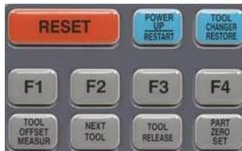
1. Locate the orange RESET key and push it to clear any alarms that are present, and to power on the servos of the machine.
