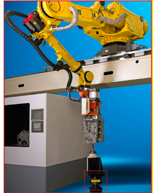
FANUC R-2000iB/165R equipped with the FANUC FS-250iA force sensor in a deburring process
