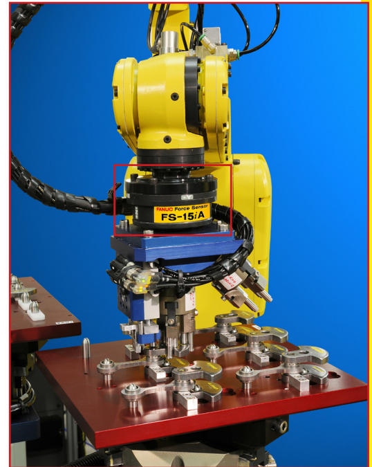
LR Mate 200iC/5L equipped with the FANUC FS-15iA force sensor performing small part assembly
