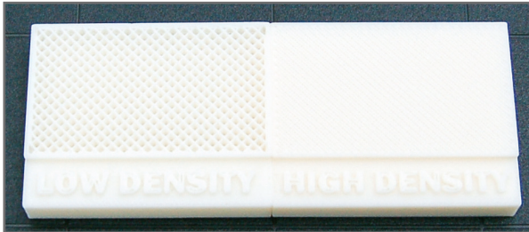
Insight software for FDM 3D Printers allows control over all build parameters, such as fill density.
