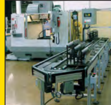
RoboFlex PT Pallet Transfer
