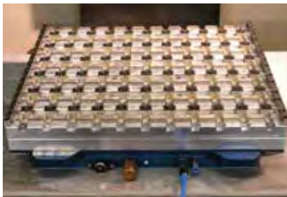
VM300 Base Unit (45175) with a Production Pallet (VM300 Blank Pallet - 45130)
