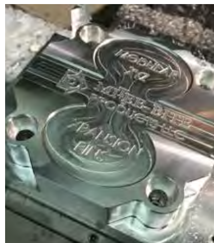
Op 2 including c'bore on same fixture
