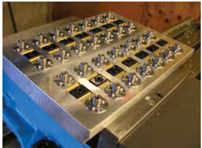
Fixtured with Mitee-Bite Machinable Uniforce® Clamps
